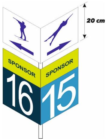
**9.1.4 T-Post / Lane Divider / Post mounted on hard wire**
